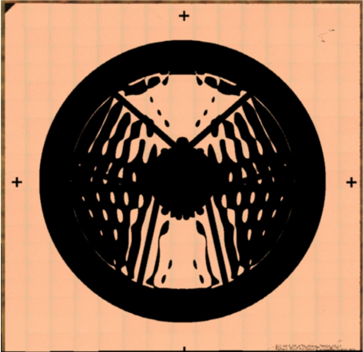
Figure 2: A downsampled version of high-resolution microscope imagery of the Milestone 2 mask, taken as part of manufacturing validation. The background lines are a stitching artifact.
