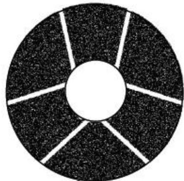
Figure 1: Approximate AFTA pupil with central obscuration and six secondary support struts.
