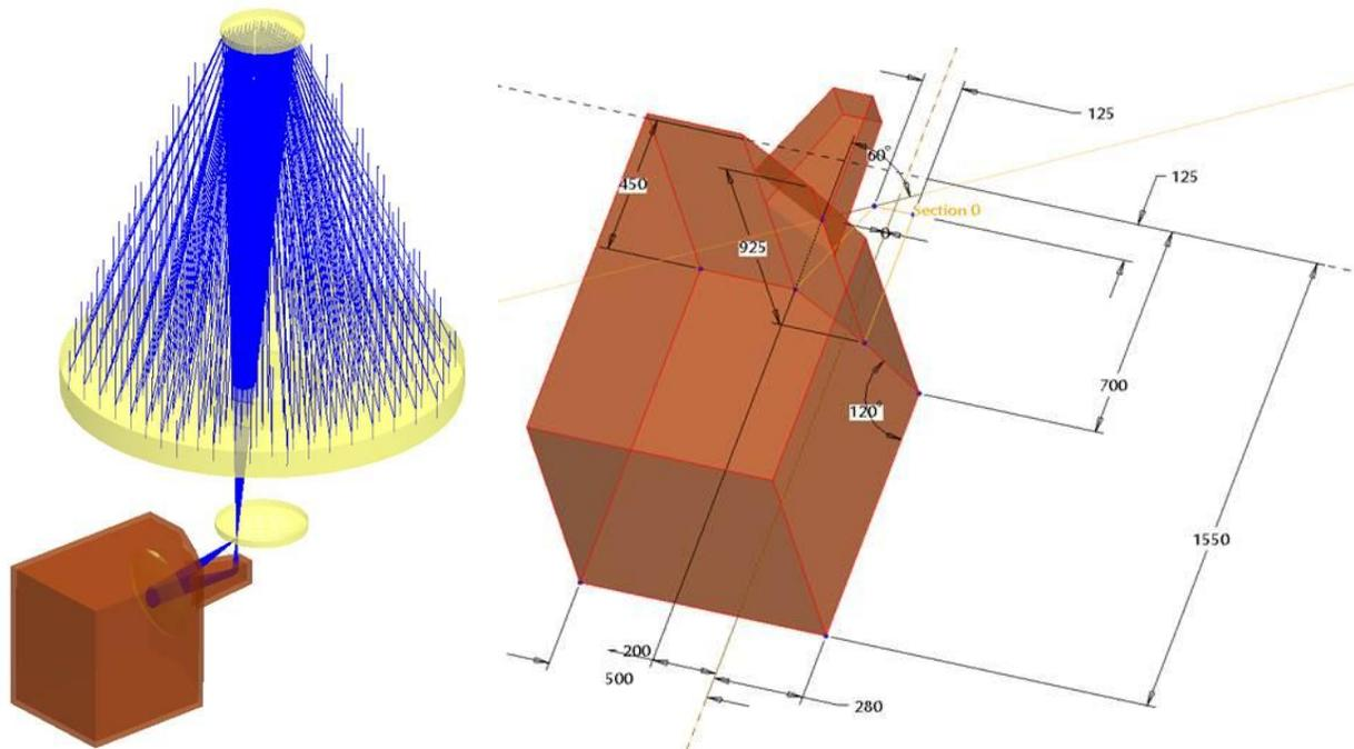
Figure 2. The box shows the coronagraph volume. The small disk behind the primary mirror indicates a 0.6 deg radius in the Cassegrain image plane.
