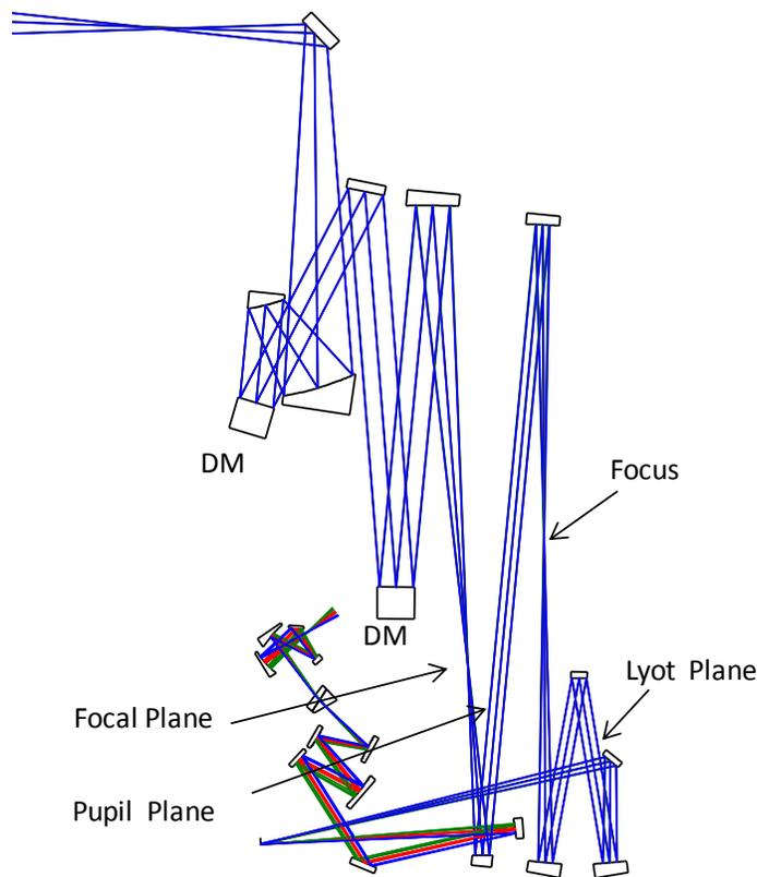
Figure 5. One additional reflection upstream of the occulter and another before the Lyot stop provide a focus following the a pupil plane. The focus can be used as a field stop to block light outside the dark hole, and it can be used as the occulter plane for a PIAA or shaped pupil coronaagraph.
