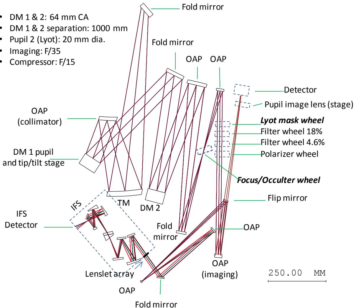
Figure 3. The coronagraph layout is for a pair of 64 x 64 mm DMs separated by 1 m of optical path. This design has only one occulter plane and one plane for a Lyot stop. It may be possible to accommodate a reflective pupil mask at the flat between the two DMs.
