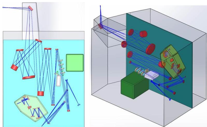
Figure 4. The instrument is shown packaged in the allocated volume. The green box represents the electronics package.
