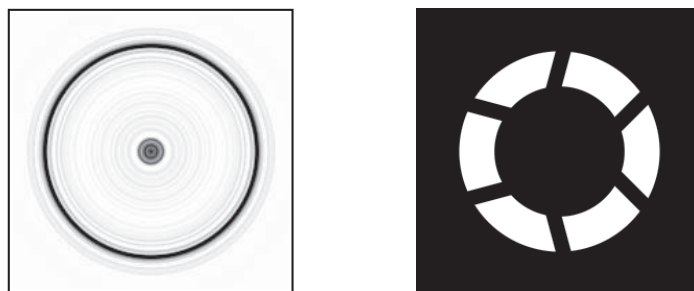
Figure 4. The coronagraph elements. At left, the metal-dielectric focal plane mask controls both the real and imaginary parts of the star's point spread function. The intensity transmittance is illustrated here. At right, pupil plane (Lyot) mask has cutouts for the central obscuration and the six support struts.
